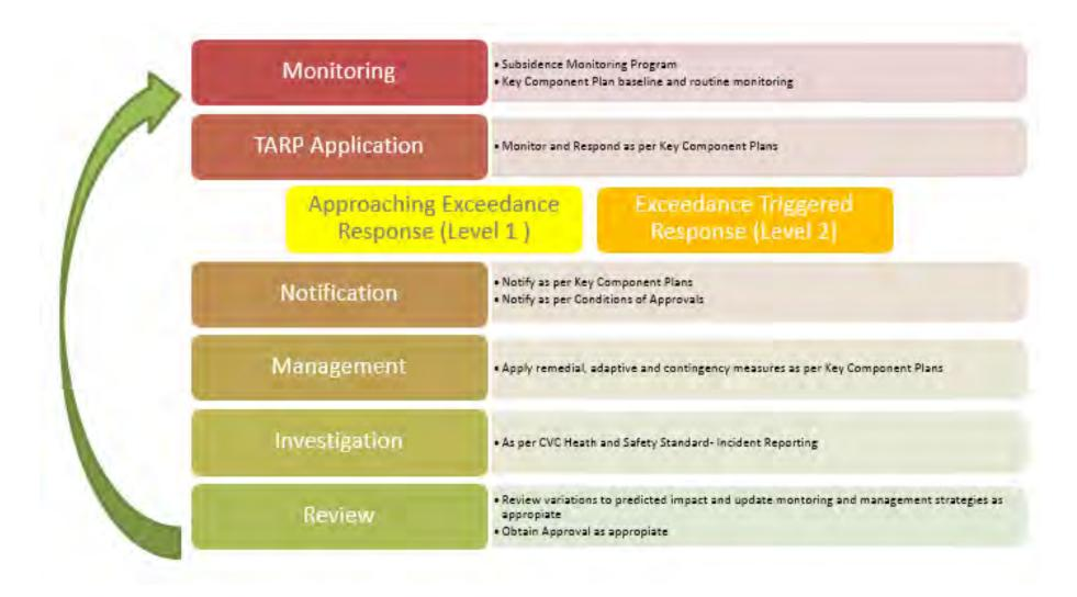
Figure 2 – Subsidence monitoring and management framework
