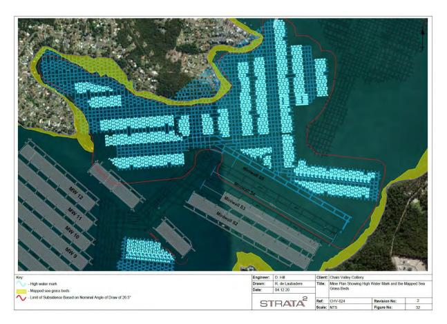
Figure 2: General underground layout and Predicted Limit of Subsidence Associated with Panels S2 and S5 and the Northern Pillar extraction area
